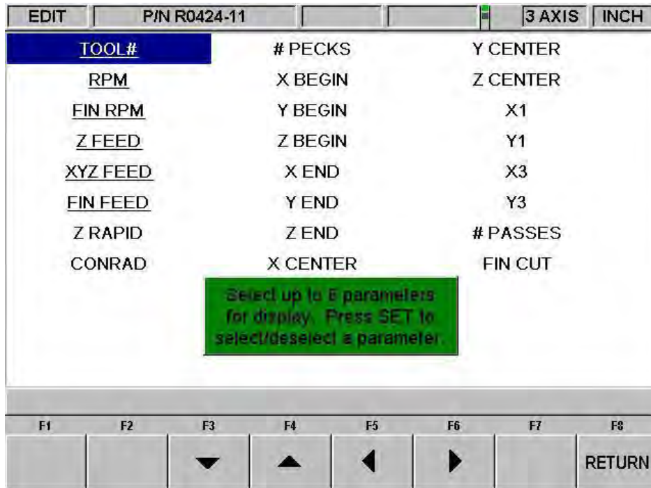
FIGURE 10.2.2 Pressing Help while viewing the spreadsheet lets you change the program parameters
